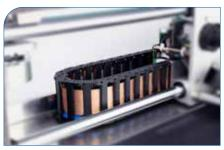
> Only one energy chain left. This can be opened on the inside. The inside separators prevent the flat ribbon cables from touching the pneumatic hose.
