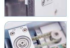
> For an easy belt replacement, the counter bearing at the brake support is removable.
