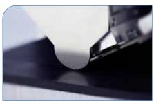
> By a folded edge, the transfer ribbon is guided around the printhead edge. This facilitates inserting the ribbon
