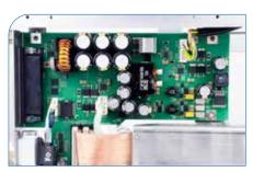
> The power electronics is now integrated in the print mechanics. Thus, it was possible to use only one cable
