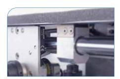
To detect the end positions, inductive sensors are now used. They are less soilsensitive.
