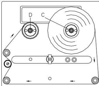
The illustration shows a left hand printing system. If you are using a right hand system, then the new roll is to be inserted at the left and the cardboard core is to be inserted at the right side.
