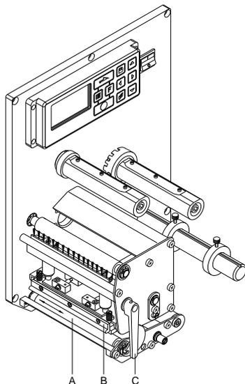
A soiled pressure roller can lead to reduced print quality and can affect transport of material.
